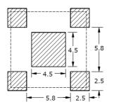
Figure 20 Recommended Soldering Footprint
