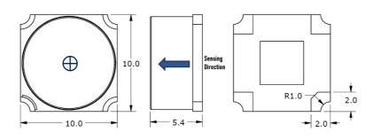
Figure 19 Outline Dimensions shown in millimeters
