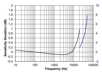
Figure 2 Typical Frequency Response
