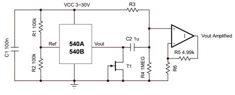
Figure 9 Typical circuit with amplifier
