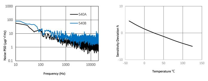
Figure 5 Noise Power Spectral Density (Noise PSD)
